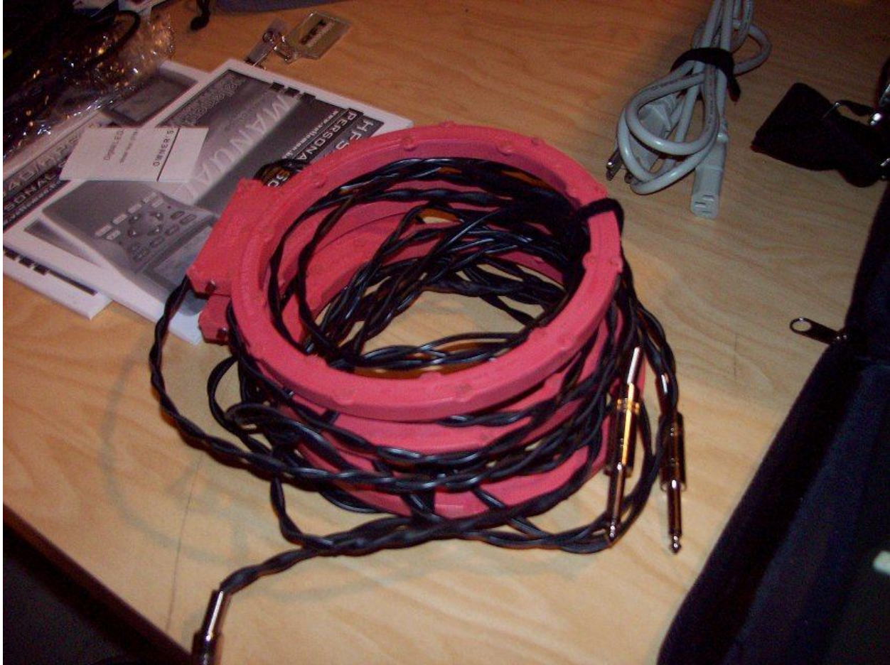
Three matching detection coils made from old TV degaussers
