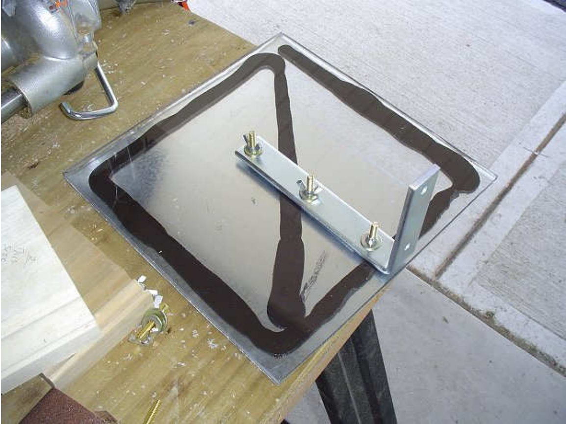
Figure 6 – Applying the adhesive between the plate and plate support
